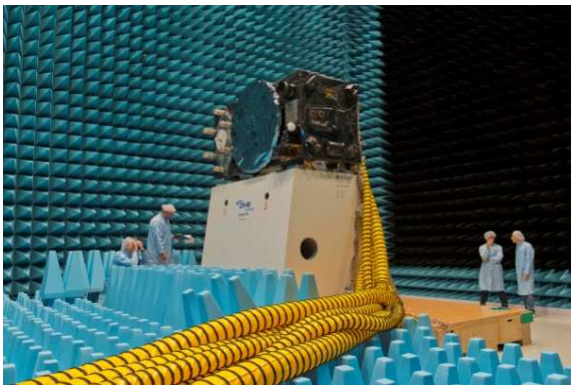
Galileo FOC-satellite being prepared for 'passive intermodulation testing' Source: ESA-Anneke Le Floc'h
